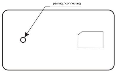
Fig. 1. Location of the pairing/connecting button
